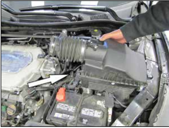
7. Lift up the air box half way out, then unhook the wiring harness from the air box and remove the air box assembly.
