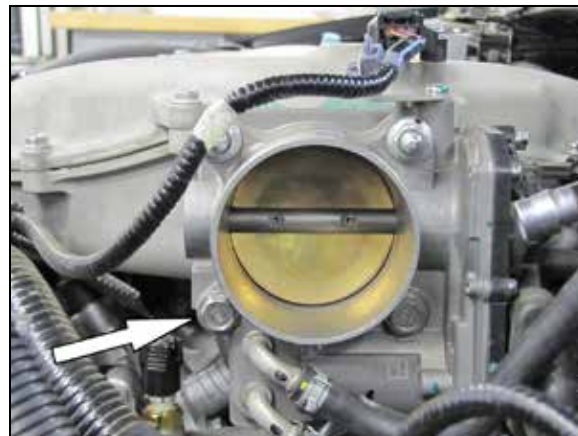
13. Remove the front lower throttle body mounting bolt. NOTE: This bolt will be reused in the next step.
