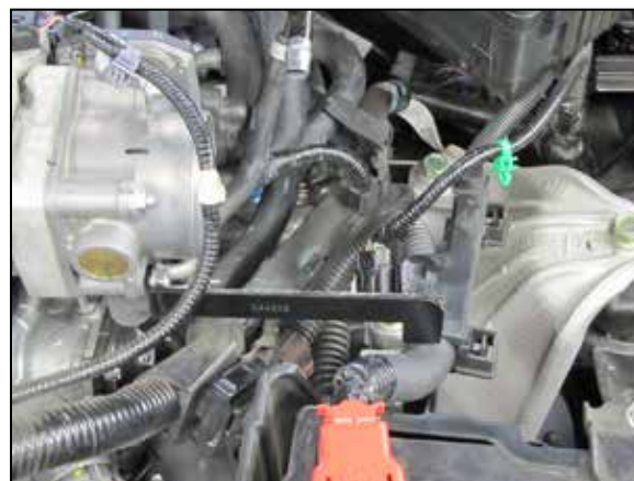
14. Install the provided tube mounting bracket (064302) onto the throttle body and secure with the factory bolt removed in the previous step.
