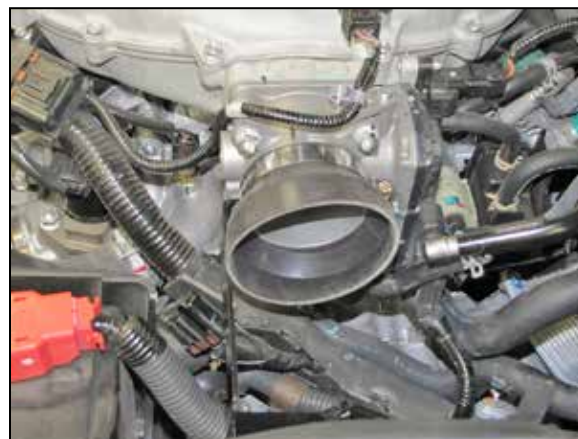
16. Install the appropriate step hose onto the throttle body and secure with the provided hose clamp. NOTE: Most Honda vehicles will use hose #084093; most Acura's will use hose #084091.
