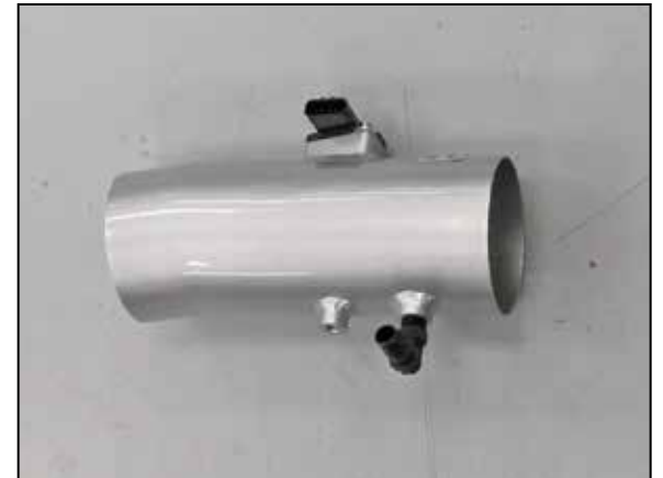
19. Install the 90° vent fitting into the K&N® intake tube as shown. NOTE: Plastic NPT fittings are easy to cross thread. Install the vent fitting "hand" tight, then turn it two complete turns with a wrench.
