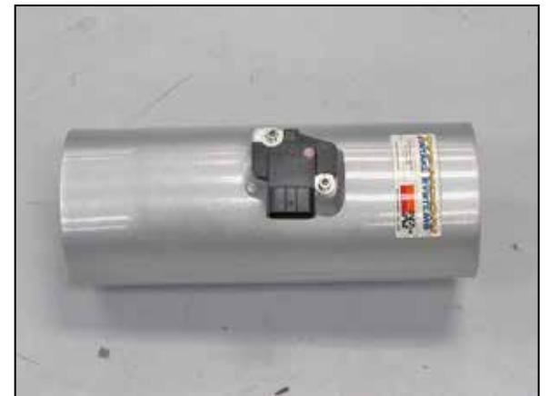
18. Install the mass air sensor into the K&N® intake tube and secure with the provided hardware.
